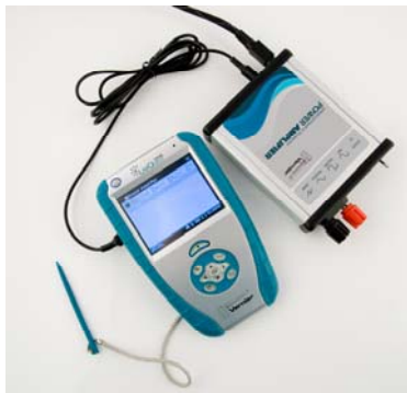
Power Amplifier connected to a LabQuest audio out connector
