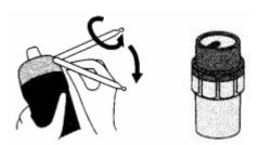
**B.** Be sure the pump handle is fully pushed in. Then insert the detector tube into the rubber inlet of the pump with the arrow (G ⇒) on the tube pointing towards the pump.
